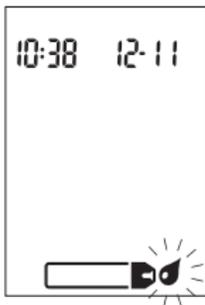
**5.** A test strip and flashing blood drop symbol appear on the display.
