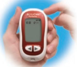
1. Press and release
