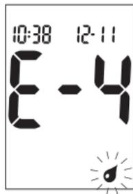
Not enough blood or control solution was drawn into the test strip for measurement or was applied after the test had started. Discard the test strip and repeat the test.
