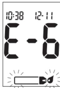
Blood or control solution was applied to the test strip before the flashing drop symbol appeared on the display. Discard the test strip and repeat the test.
