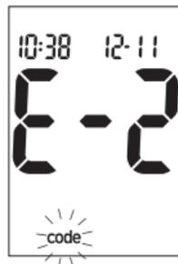
The code chip is incorrect. Turn off the meter and insert a new code chip. If this does not fix the problem, call Roche.
