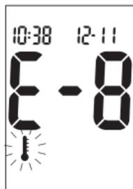
The temperature is above or below the proper range for the meter. Refer to the test strip package insert for system operating conditions. Move to an area with the appropriate conditions, wait five minutes and repeat the test. Do not artificially heat or cool the meter.
