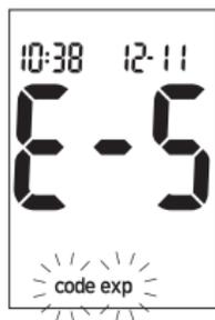
The code chip is from an expired lot of test strips. Ensure the code chip number matches the code number on the test strip container. Make sure the time and date in the meter are correct.
