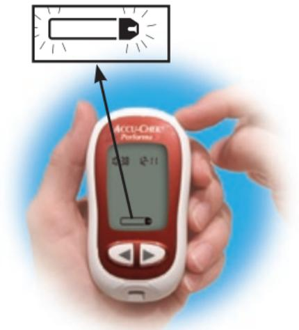
5. To set up more options, press and release ⓪. To exit, press and **hold** ⓪ until the flashing test strip symbol appears on the display.
