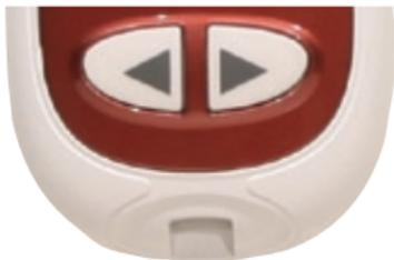
4. Press and release ◀ or ▶ to switch between “On” and “OFF.”
