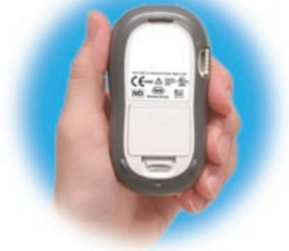
4. Turn the code chip over so the code number faces down. Push the code chip into the code chip slot until it stops.
