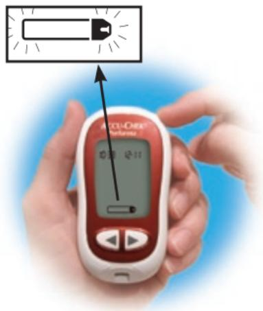
1. Press and release
