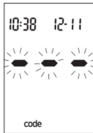
The meter is not coded or the code chip is not inserted. Turn off the meter and recode it.
