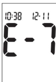
An electronic error occurred or, in rare cases, a used test strip was removed and reinserted. Turn the meter off and on, or take the battery out for 20 seconds and reinsert it. Perform a blood glucose or control test. If the problem persists, call Roche.
