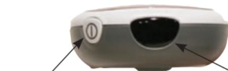
**On/Off/Set Button****Top View****Infrared (IR) Window**
