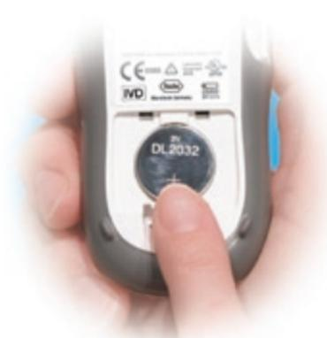
1. Open the battery door on the back of the meter by pushing the tab in the direction of the arrow and pulling the door up. Remove the old battery.
