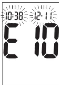
The time and date settings may be incorrect. Make sure the time and date are correct and adjust, if necessary.
