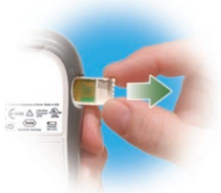
3. Remove the old code chip (if there is one in the meter) and discard it.
