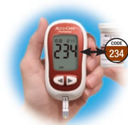
1. Insert the test strip into the meter in the direction of the arrows. The meter turns on.
