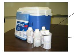
Place the requisition form in the plastic bag, and wrap the plastic bag around the bottle with the elastic band
